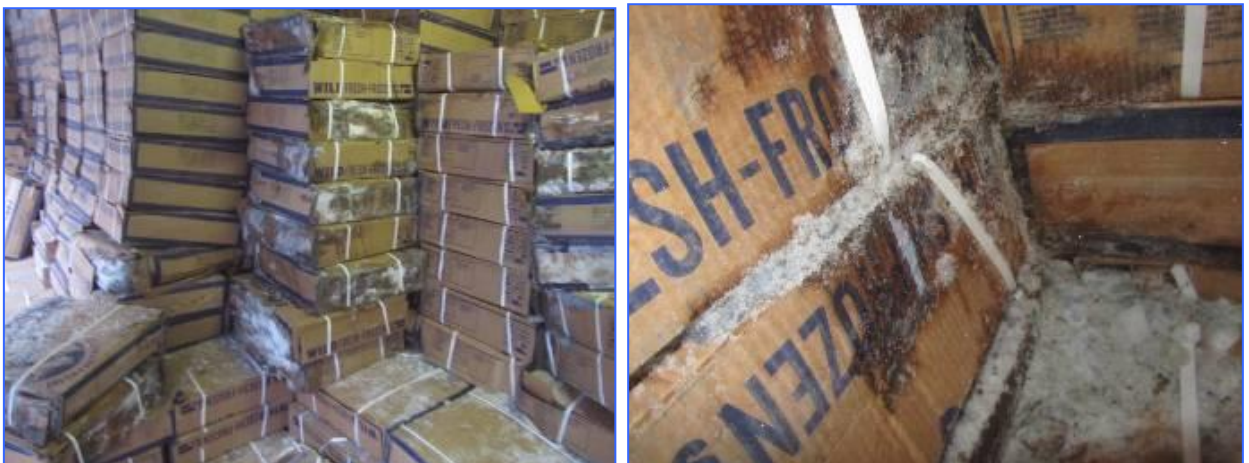
Photos illustrating packaging damage, caused by high moisture during cargo handling operations.
