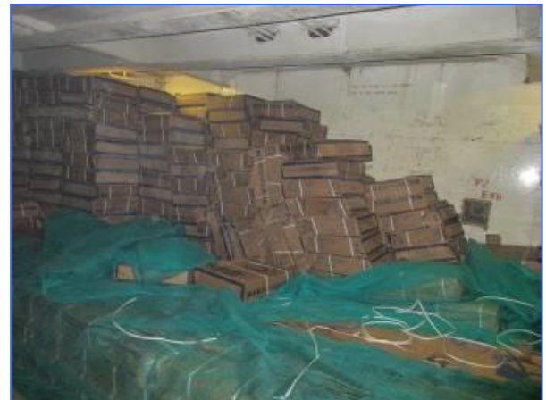
Photos illustrating separation of the cargo by thin fiber nets.
